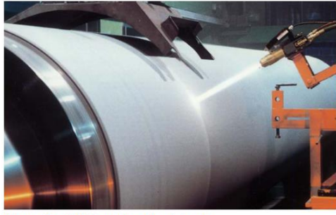
Figure 22 • HVOF coating of a sink roll
